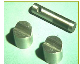
After ASTM D 2670 Wear Test
