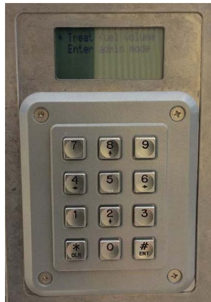
On board 12-24V dosing system
