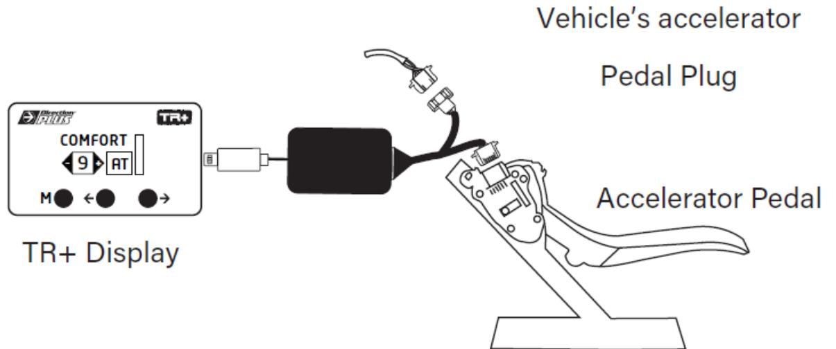
1. Disconnect the plug from the Accelerator Pedal (be aware of any locking clips that maybe present).
